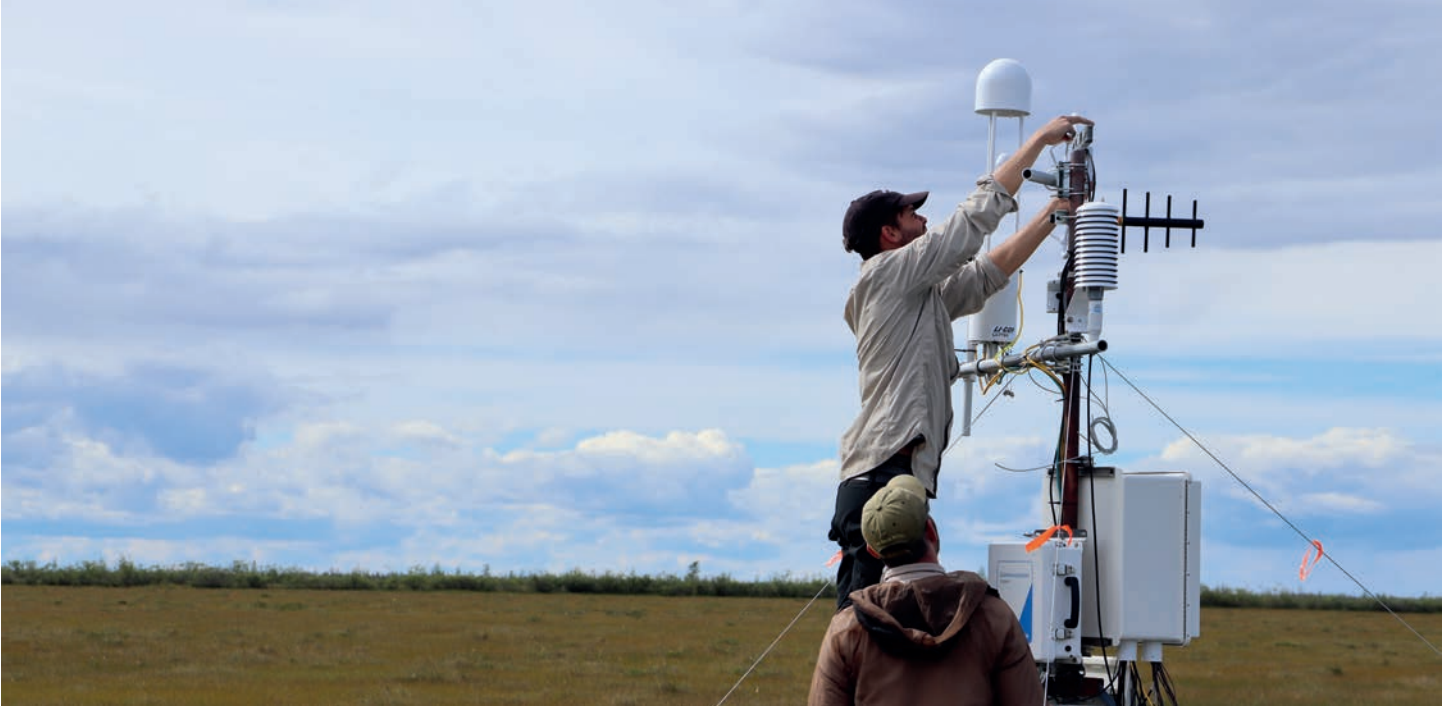
Woodwell's Dr. Kyle Arndt and Patrick Murphy installing an eddy covariance flux tower in Churchill, Manitoba, Canada — the inaugural new tower of the Permafrost Pathways project.
