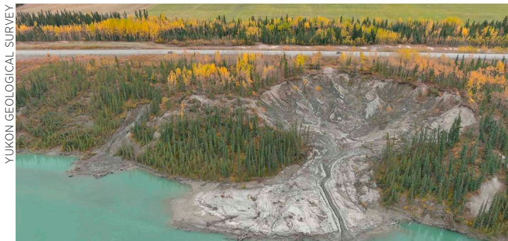
A permafrost thaw slump threatens a highway near Whitehorse, Yukon.
