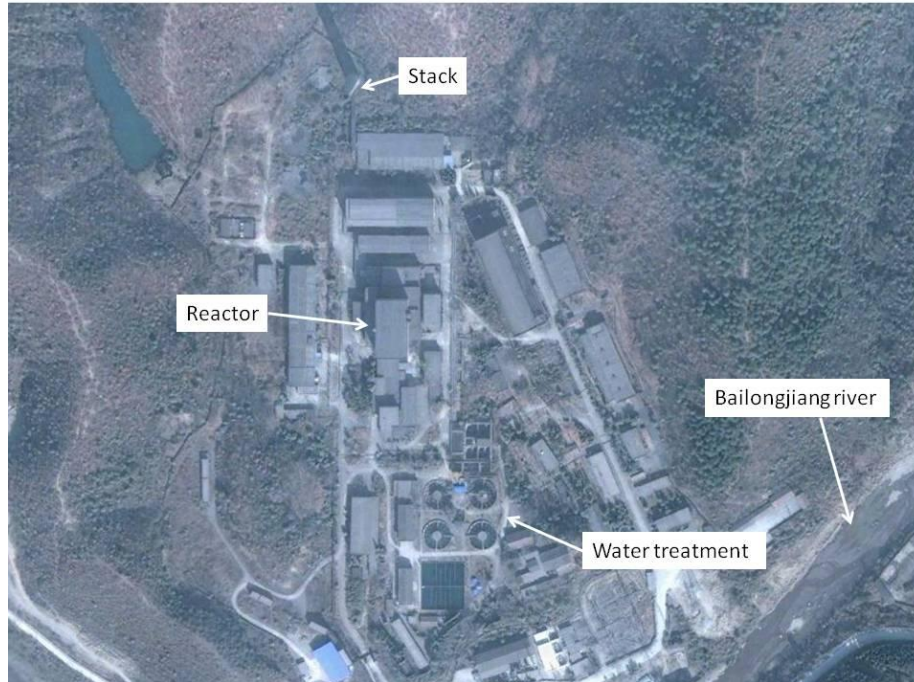
Figure 4: The Guangyuan plutonium production reactor.
